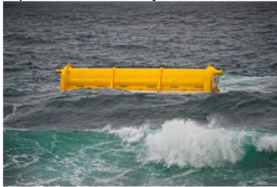
Oscillating wave surge convertor Aquamarine Power Oyster
