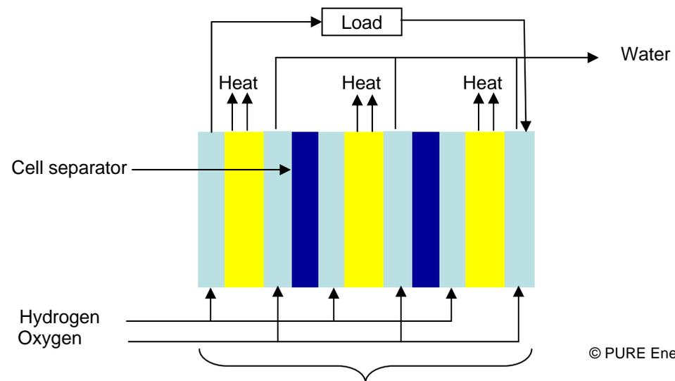
A fuel cell stack (several single fuel cells in series)
