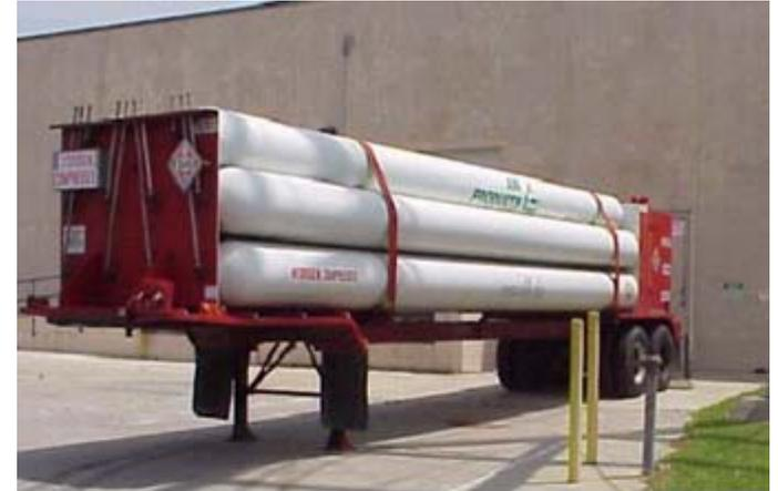
(Above) Hydrogen tube trailer containing approximately 300kgH<sub>2</sub>. Source: Air Products
