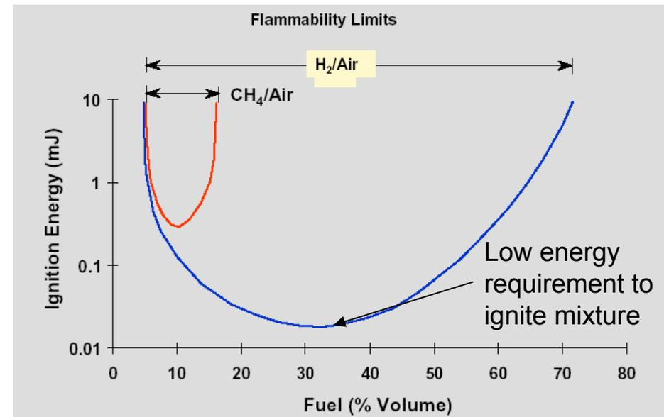
The range of flammability of H<sub>2</sub>/air mixtures is wide. However the lower limit, which is normally most important (i.e. the point at which the mixture first becomes flammable) is similar to that of a methane/air mixture.
