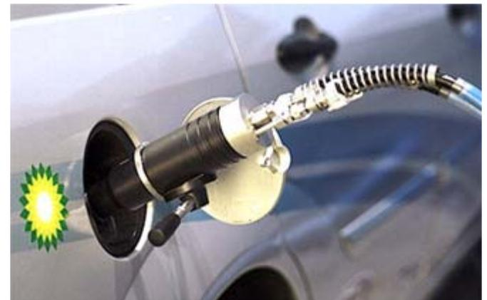
Connection of a hydrogen dispenser nozzle for filling with compressed hydrogen
