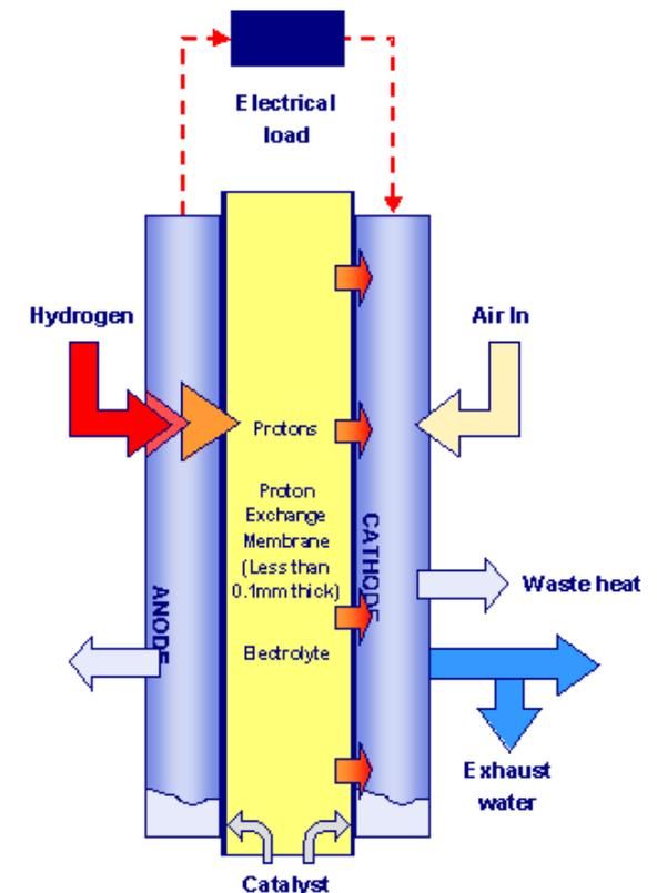
Cross section through a typical fuel cell
