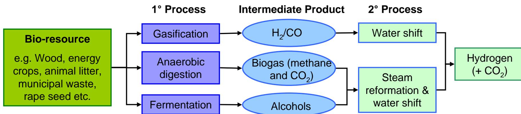
**Gasification** is a relatively well-known technology for the generation of hydrogen from heavy hydrocarbons at a large-scale and is being developed as an option for the treatment of municipal solid waste (MSW). However small-scale biomass gasifiers are rare and the technology is still undergoing substantial R&D. The hydrogen produced by small-gasifiers usually requires extensive clean-up before it can be used in a fuel cell, or even gas engine.
