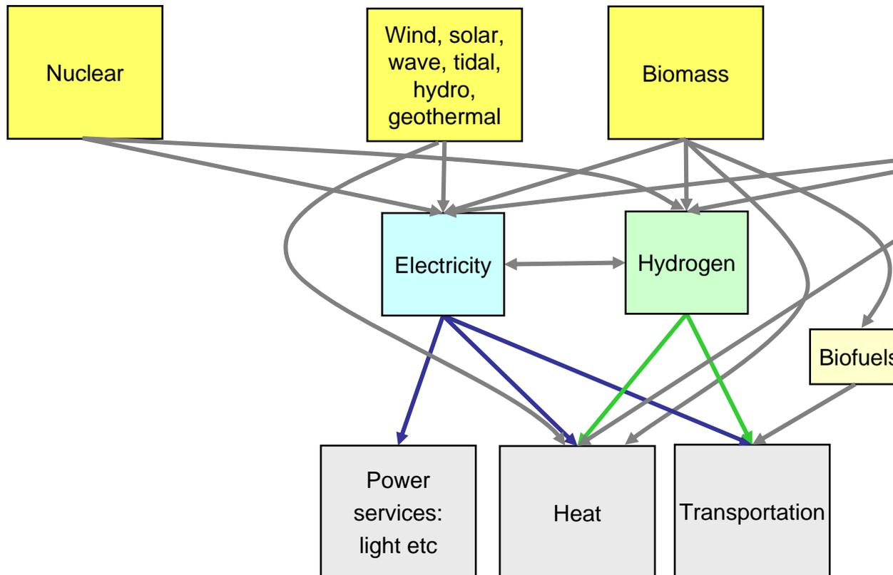
Following the arrows from energy source to end-use in this diagram defines an 'energy chain'.
