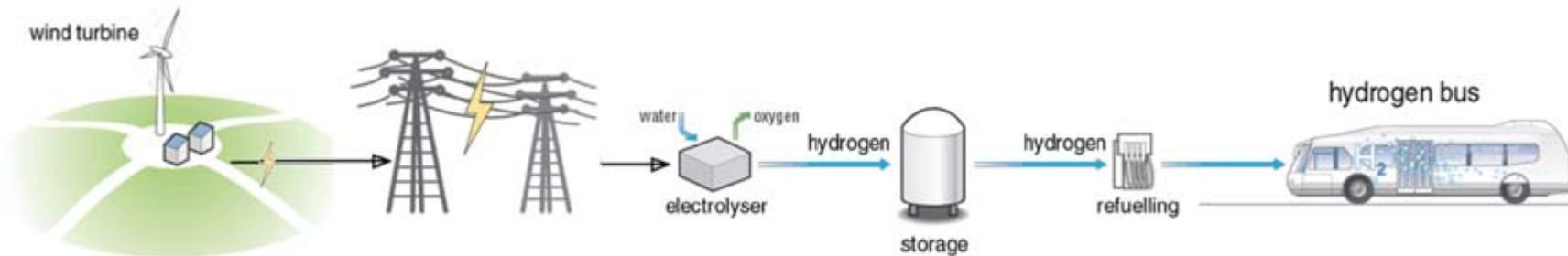
The image above is a simplified example of a renewable hydrogen project. A primary energy source (in this case, electricity from a wind turbine) is fed into an electrolyser, which is a device for generating hydrogen. The hydrogen is then compressed and stored before being sent to a refuelling dispenser. In the example above, a hydrogen powered bus defines the end of the chain. In general, however, the hydrogen may be also used to generate electricity, or heat.
