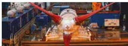
Installation of the Hammerfest Strom Tidal Turbine at the test site at Eday, Orkney
